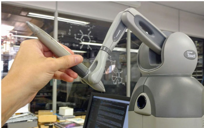
FIGURE 3.7: Geomatic Touch Phantom haptic device used in the nanomanipulation application. The arm is able to register pose in 3D space with 6 degrees of freedom (DOF) and generating forces on the end effector (pen's point) with 3 DOF (X, Y and Z).
