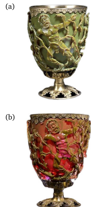
FIGURE 1.1: (a) Lycurgus cup when illuminated from the front and (b) when illuminated from the back (adapted from [2])
