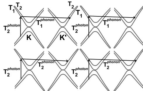
FIG. 6. The four allowed DRR processes in bilayer graphene, taking into account the optical anisotropy.
