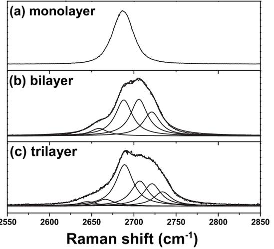
FIG. 5. The measured Raman spectra of the  $G'$  band of a (a) monolayer, (b) bilayer, and (c) trilayer graphenes. The samples were made by exfoliating graphite on top of a 100 nm silicon oxide substrate using 2.41 eV laser energy. The  $G'$  band for monolayer, bilayer, and trilayer graphenes were fitted with one, four, and six Lorentzians, respectively, with a FWHM of  $24 \text{ cm}^{-1}$ .
