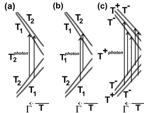
FIG. 3. [(a) and (b)] Schematic electron dispersion of bilayer graphene along the  $K\Gamma$  direction showing the possible transition induced by (a) a photon with  $T_2$  symmetry ( $x$  polarization) and (b) a  $T_1$  photon ( $y$  polarization). (c) The electronic dispersion of trilayer graphene showing the five possible transitions induced by light absorption.
