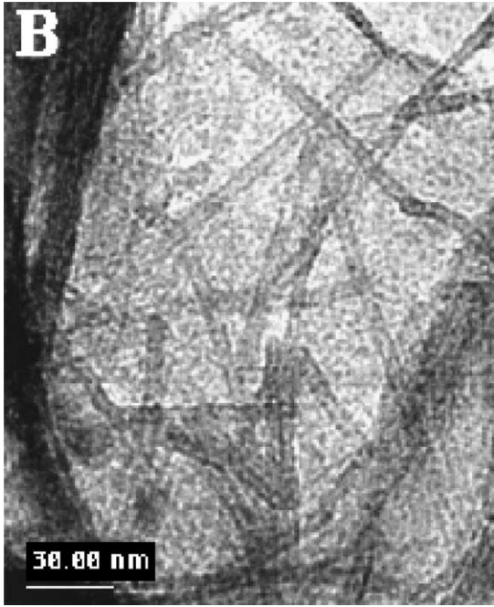
Fig. 3. A transmission electron microscope image of bismuth nanotubes. The X-ray diffraction pattern shows that bismuth nanotubes have the same space group R\bar{3}m(166) as bulk bismuth with similar lattice constants [15].
